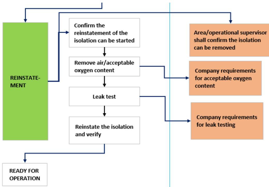
Figure 8 Subsidiary steps in reinstating the equipment/system.
