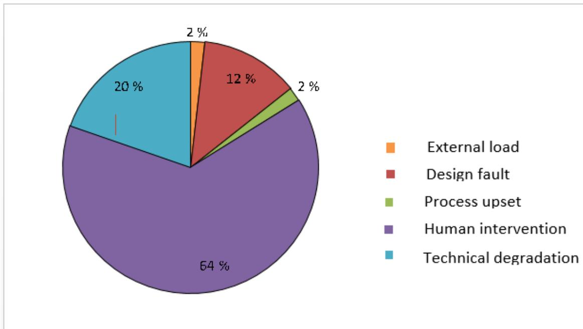
Figure 3 Reasons for hydrocarbon leaks greater than >0.1 kg/s.
