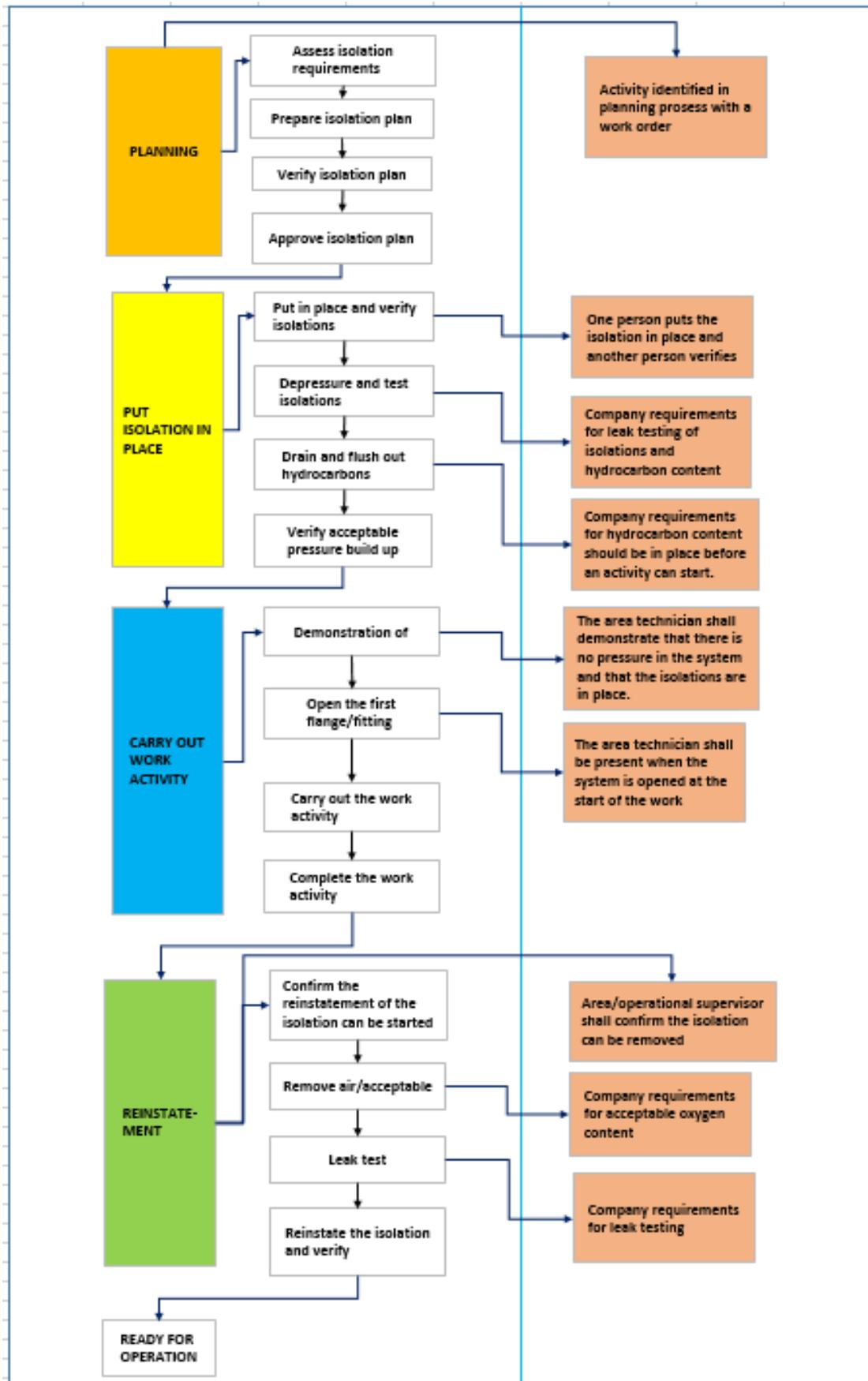
Figure 4 Flow diagram for isolation.
