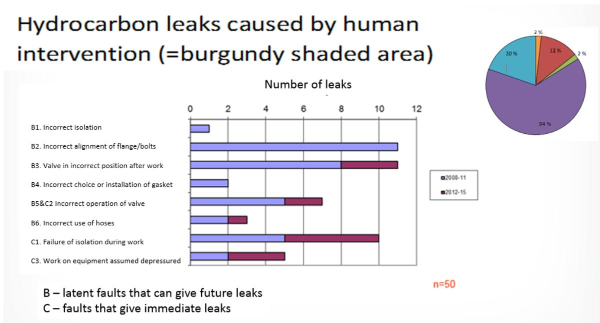
Figure 2 HC leaks in connection with manual intervention.
