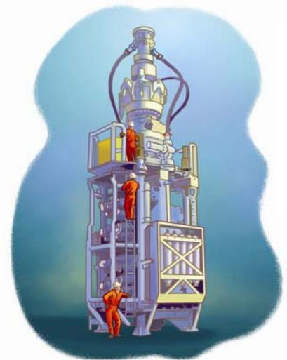
*The blow out preventer consists of 3-5 large valves that can be closed so that oil and gas cannot flow to the surface.*
