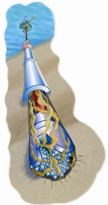
*The drilling mud keeps the pressure in the reservoir under control, and prevents oil and gas from penetrating into the well.*
